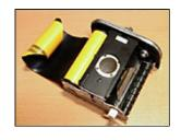
Pull the leader back and across the the magazine's pressure plate. Make sure that the colored side of the leader is against the pressure plate, and the black side is facing away, or toward you, and the edge of the paper is under the chrome lip at the edge of the pressure plate. (red arrow)
